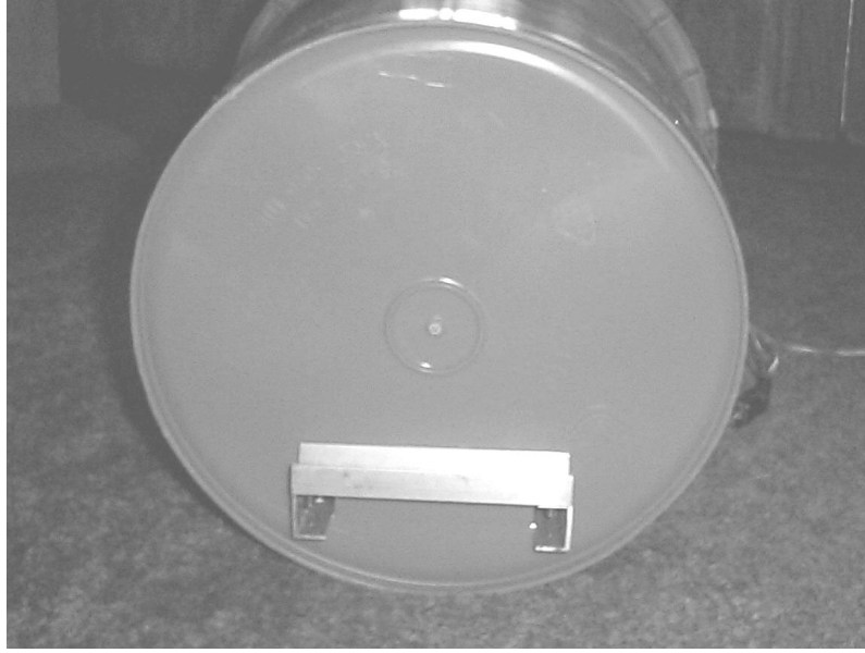
Figure 10: Retainer bracket at rear of feed bucket
