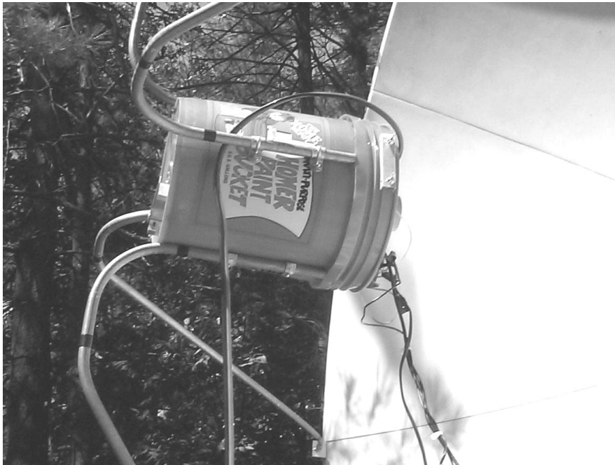
Figure 9: The Feed Bucket (Note the name of the manufacturer/equipment-vendor on the side). The bucket contains a 3.456GHz transverter in this picture.
