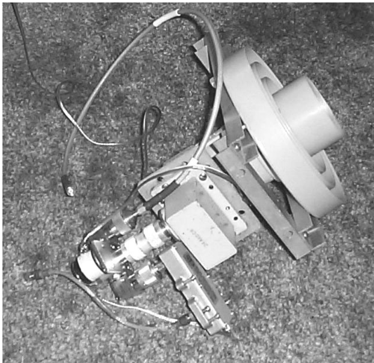
Figure 12: Chaparral feed, waveguide transition, relay, and RF pre-amplifier in mounting frame
