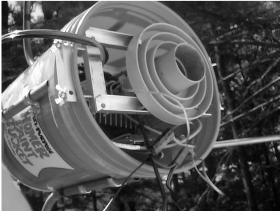
Figure 13: Transverter, feed, and amplifiers for 3.456GHz Mounted in the feed bucket
